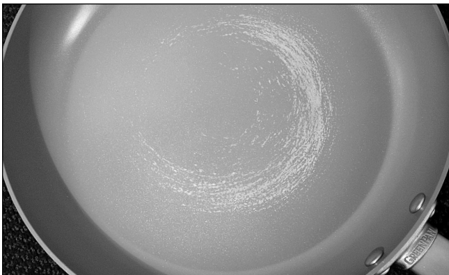
Severe damage to the interior of a ceramic-coated GreenPan after 11 cycles of the "Tiger Paw" cooking test. Pans coated with Whitford's normal nonsticks typically reach 60-65 cycles before showing similar wear.
