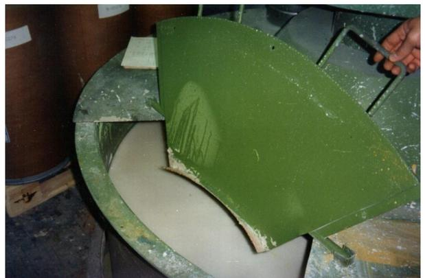
Mixing vessel for paint,
