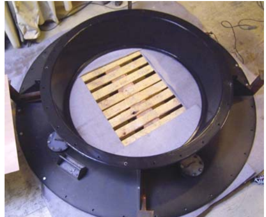
Large ring ø 2.2 m coated with Accopon HBA
