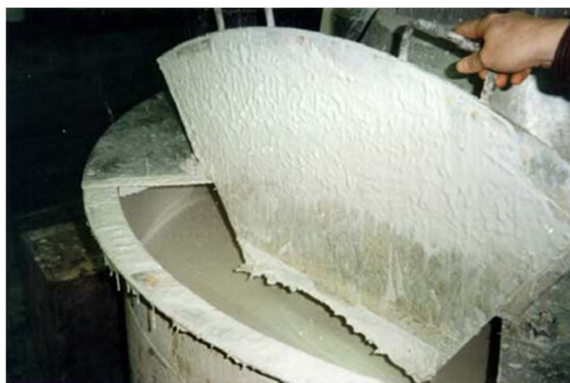
Paint vessel without coating
